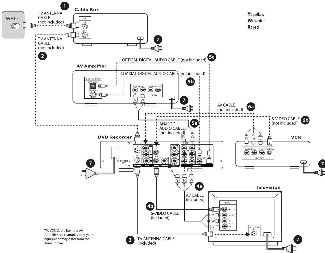
1. Connect a TV antenna cable from your wall outlet to your cable box.
