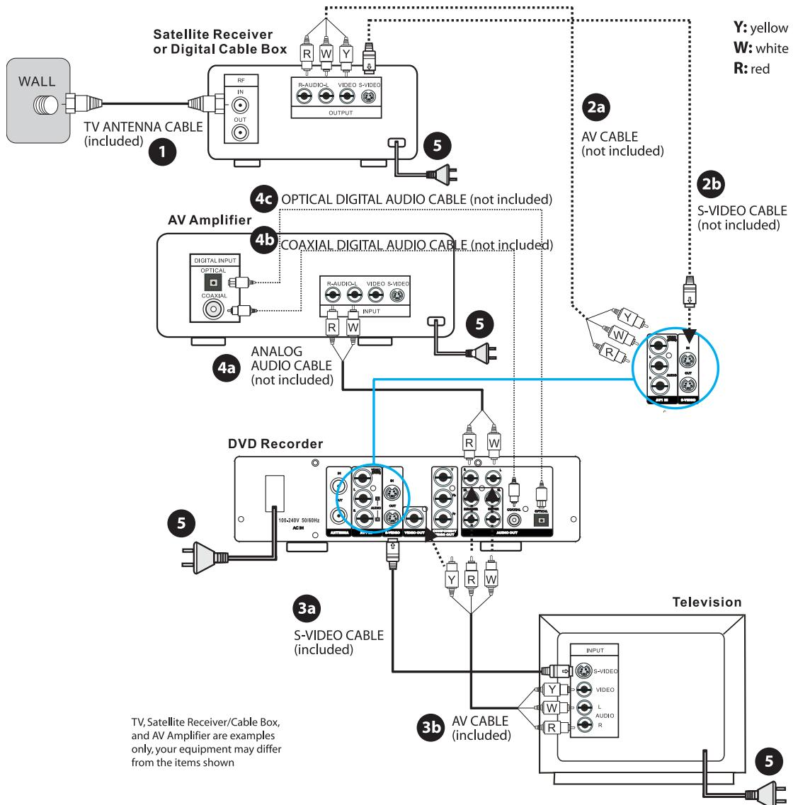
1. Connect a TV antenna cable from your wall outlet to ANTENNA IN on the DVD recorder.
