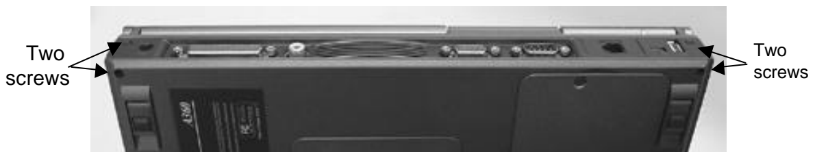
Figure 5-9 Four Screws Securing the LCD Hinges
