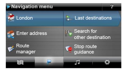
All of the software functions are organised in hierarchical menus which are called up by pressing the buttons on the touchscreen of your navigation device. Each button opens up the level underneath, which then provides access to other options relevant to this menu or function. If a button has not been assigned to another menu level, the function is performed directly.
