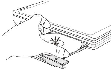
4. Test that the disc is able to turn freely and then push the tray back into the optical drive carefully.
