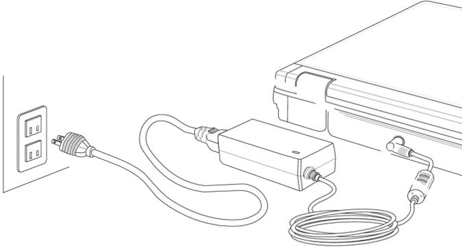
The adapter provides the notebook with power and also charges the battery. The power supply indicators of the notebook provide details on the operating state. The battery is also being charged when you are working on your notebook with the power adapter. The power adapter is still live if the notebook is not connected with it. You should therefore unplug the power adapter from the outlet if it is not connected to the notebook.
